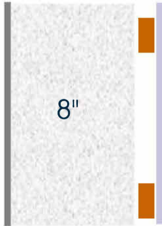
STC 47 1/8" PC on 8" AAC4 1-1/4" Furring Gyp. Board
