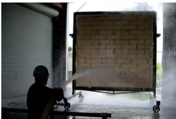
AAC Block wall PASSES Hose Stream Test
