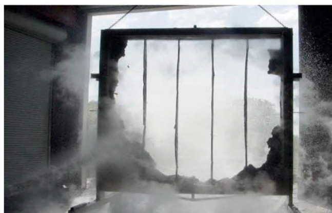
Gypsum Board Wall FAILS Hose Stream Test
